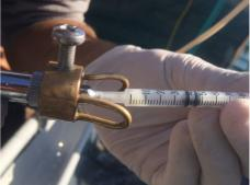
Picture 7: Calibration with 1ml syringe
